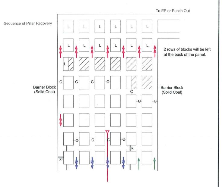
Blocks on the bleeder side of the section will be mined from one side only for ventilation purposes.
