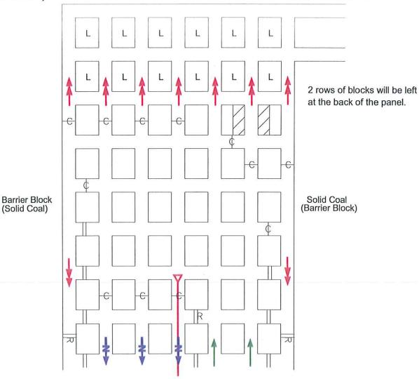
Blocks on the bleeder side of the section will be mined from one side only for ventilation purposes.
